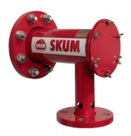
SKUM tank protection hardware is designed for effective suppression of most flammable liquid hazards and is primarily constructed of high-quality 316L stainless steel and/or zinc-free bronze materials. Quick control of a flammable liquid storage tank fire is critical to minimise structural damage and protect tank contents. SKUM hardware offers protection for cone, fixed, open, closed, or floating roof designs, vertical or horizontal tanks, hydrocarbon or polar solvent hazards.
